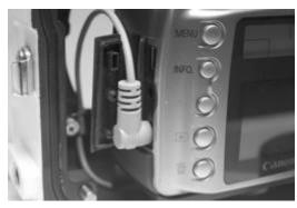
Picture B: Trigger release cable position
